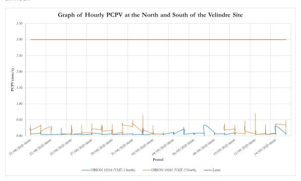
No vibration data recorded exceeded the 1.00mm/s limit at both the North and South monitoring stations on the Velindre site in the period 21/08/2025 -15/09/2025.
