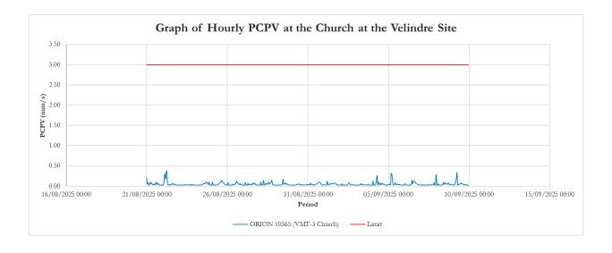
No vibration data recorded exceeded the 1.00mm/s limit at the Church monitoring station outside the Velindre site for the period covering 21/08/2025 – 09/09/2025.
