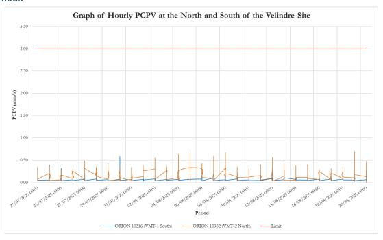
No vibration data recorded exceeded the 1.00mm/s limit at both the North and South monitoring stations on the Velindre site in the period 23/07/2025 – 20/08/2025
