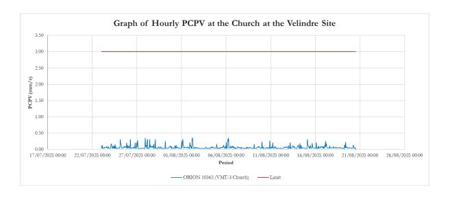
No vibration data recorded exceeded the 1.00mm/s limit at the Church monitoring station outside the Velindre site for the period covering 23/07/2025-20/08/2025
