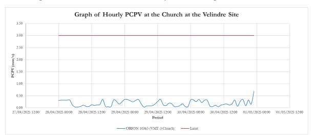
No vibration data recorded exceeded the 1.00mm/s limit at the Church monitoring station outside the Velindre site for the period covering 28/04/2025-27/05/2025.
