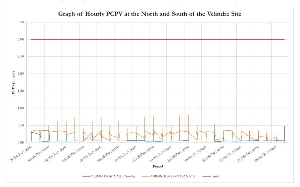
No vibration data recorded exceeded the 1.00mm/s limit at both the North and South monitoring stations on the Velindre site for the period covering 28/04/2025-27/05/2025.
